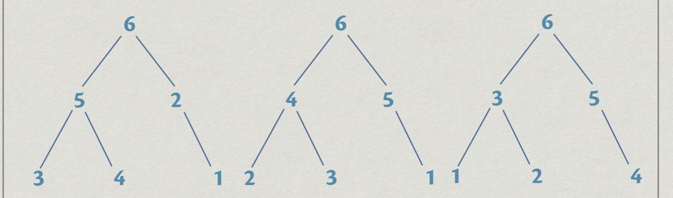
In a heap, the largest element is always at the root
