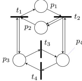
Figure 2: Example of a Petri net with progressive transitions
