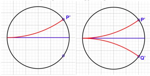
The point P' is the transformation of P, and the colour codes give the rest. The point is this, since the blue line meets the black circle at right angles, it must be a diameter. The lower half of the black circle is the transformation of the diameter
