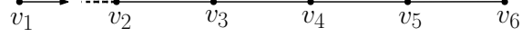
Figure 2: An example of a generalized witness to disconnectedness, where only a BFS from v_1 (but not from any other vertex) detects the generalized witness.
