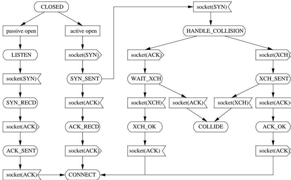
Fig. 3. An enhanced connection protocol
