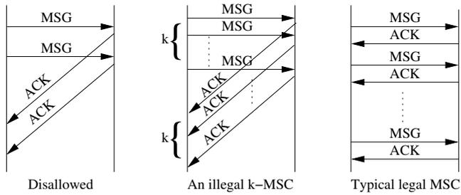
Fig. 7. MSC specifications for the counting process
