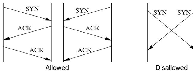
Fig. 2. MSC specifications for the connection establishment protocol
