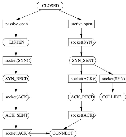
**Fig. 1.** A simple TCP-like connection establishment protocol
