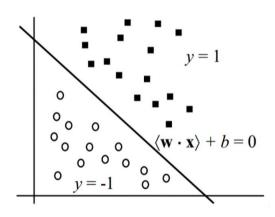
■ Dot product  $w \cdot x$  $\langle w_1, w_2, \dots, w_n \rangle \cdot \langle x_1, x_2, \dots, x_n \rangle = w_1 x_1 + w_2 x_2 + \dots + w_n x_n$
