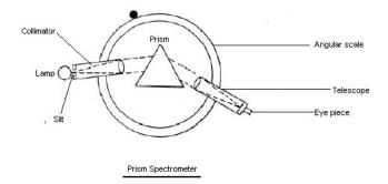
• First the telescope has to be focussed distant objects i.e infinity and this has to be maintained until the experiment is over, so as not to refocus again. Then, the cross-wires should be focussed by moving the eye-piece of the telescope.
