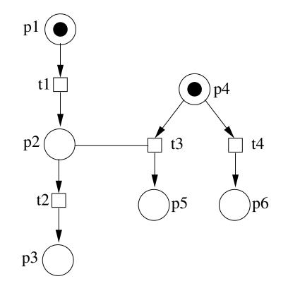
$t_2$  and  $t_3$  are in a special relation; no conflict in the usual sense, since both can happen, but  $t_3$  must happen first.
