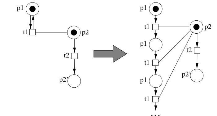
The set C' of all transitions in the unfolding fulfils conditions (i) and (ii) but not (iii). Indeed, there is no firing sequence containing all transitions in C' – when would one fire  $t_2$ ?
