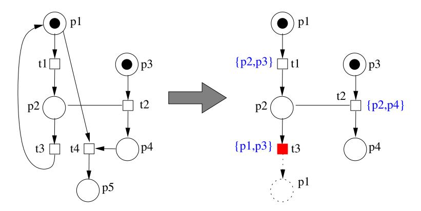
The occurrence of  $t_3$  in the unfolding is declared a cut-off; therefore,  $t_4$  is never added (even though  $t_1 t_2 t_3 t_4$  can be fired in the net).
