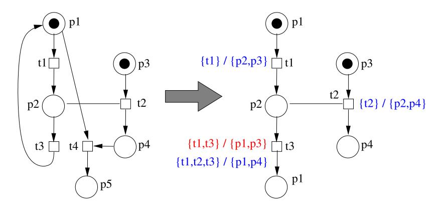
Notice that the pair  $\langle t_3, \{t_1, t_2, t_3\} \rangle$  is *not* a cut-off!
