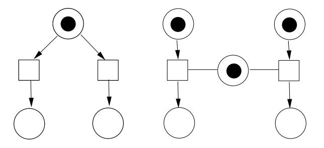
Different concurrent semantics (no difference for interleaving semantics). Same set of reachable markings. Here, we are interested in their unfoldings. For **bounded** nets, the reachability graph is finite.
