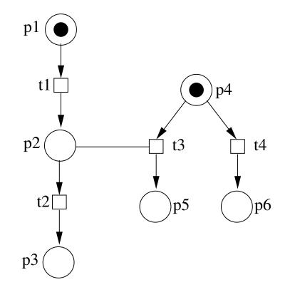
This notion generalizes causality and (symmetric) conflict, i.e. we have  $t_1 \nearrow t_2$ ,  $t_1 \nearrow t_3$  (causes),  $t_3 \nearrow t_2$  (asymm. conflict),  $t_3 \nearrow t_4$ , and  $t_4 \nearrow t_3$  (normal conflict).
