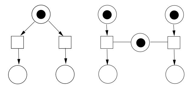
Intuition: The read arc does not consume or touch the token, it merely verifies its presence. For any transition t, we distinguish its preset  $\bullet t$ , its context  $\underline{t}$ , and its postset  $t^{\bullet}$ .
