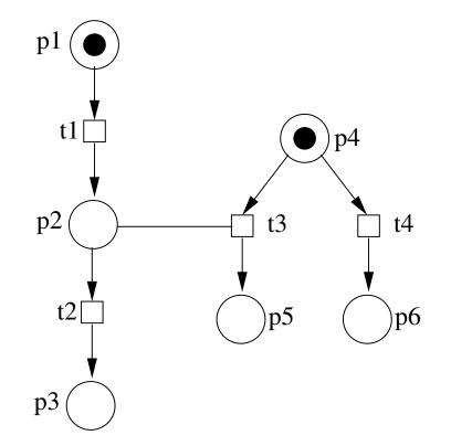
Let us re-formulate x < y as "x must necessarily occur before y." Then we have (as usual)  $p_1 < t_1$  and  $t_1 < p_2$ , but also  $t_1 < t_3$ .
