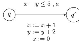
The transition from  $q$  to  $q'$  has the diagonal guard  $x - y \leq 5$ . Once the transition is taken, the value of  $x$  is increased by 1 from its current value, the value of  $y$  is increased by 2 and the value of  $z$  is set to 0 (the normal reset). More formally, each transition is of the form  $(q, a, g, R, q')$  where  $R$  is a function that maps each clock  $x$  to either 0 or  $x + c$ , where  $c \in \mathbb{N}$ .
