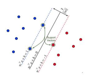
Minimize  $\frac{|w|}{2}$ Subject to  $w_1 x_1^i + w_2 x_2^i + \cdots + w_n x_n^i + b > 1, \text{ if } y_i = 1$  $w_1 x_1^i + w_2 x_2^i + \cdots + w_n x_n^i + b < -1, \text{ if } y_i = -1$
