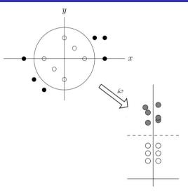
• *K* is a kernel for transformation  $\varphi$  if  $K(x, z) = \varphi(x) \cdot \varphi(z)$
