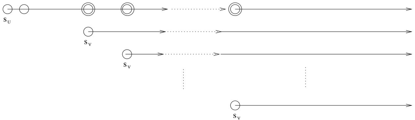
The top line is the “run” of  $A_U$  on  $\sigma$ . Note that at every prefix where  $A_U$  enters an accepting state, a new copy of  $A_V$  is started off. As it stands, this construction is not finite state as there may be even infinitely many prefixes of  $\sigma$  in  $U$  and so there would be unboundedly many copies of  $A_V$ .
