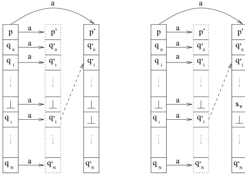
In the picture above, the left handside illustrates a move when  $p' \notin F_U$  and the right handside illustrates the case when  $p' \in F_U$ . Note, how  $q'_i$  is replaced by  $\perp$  since  $q'_i = q'_1$ . The run of the copy of  $A_V$  at coordinate  $i$  has been “handed over” to copy at coordinate 1. We shall refer to this as  $i$  merges with 1. Observe that whenever  $i$  merges with  $j$ ,  $i > j$ .
